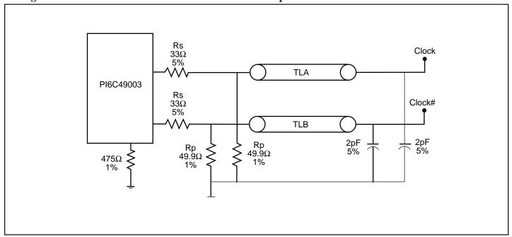
Figure 4. Configuration Test Load Board Termination
