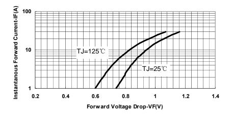
Fig.3-Typical Forward Voltage Drop Characteristics
