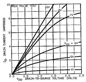
Fig. 2 - Typical Output Characteristics
