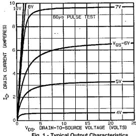
Fig. 1 - Typical Output Characteristics
