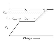
Fig. 13a - Basic Gate Charge Waveform
