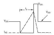
Fig. 12b - Unclamped Inductive Waveforms
