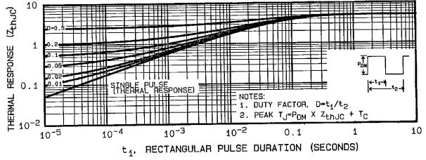
Fig. 11 - Maximum Effective Transient Thermal Impedance, Junction-to-Case
