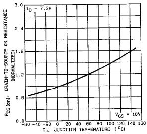
Fig. 4 - Normalized On-Resistance vs. Temperature
