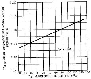
Fig. 10 - Breakdown Voltage vs. Temperature
