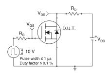
Fig. 10a - Switching Time Test Circuit
