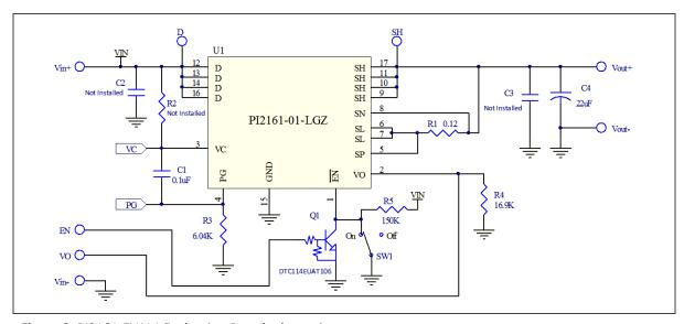
Figure 2: PI2161-EVAL1 Evaluation Board schematic.
