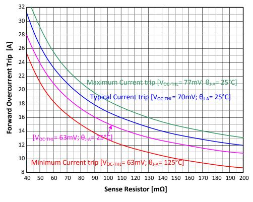
Figure 3: PI2161 Overcurrent trip vs. sense resistor chart
