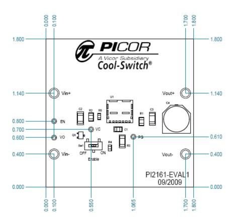
Figure 8: PI2161-EVAL1 evaluation board mechanical drawing.
