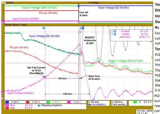
Figure 5: Plot of PI2161 response time to a forward over-current condition
