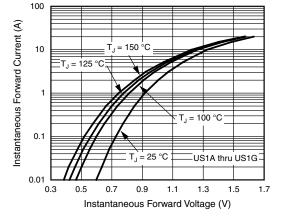
Fig. 3 - Typical Instantaneous Forward Characteristics
