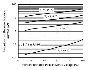
Fig. 4 - Typical Reverse Leakage Characteristics
