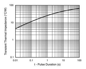
Fig. 8 - Typical Transient Thermal Impedance
