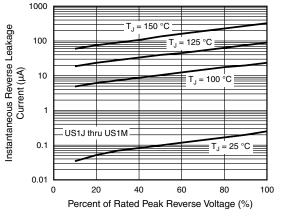
Fig. 6 - Typical Reverse Leakage Characteristics
