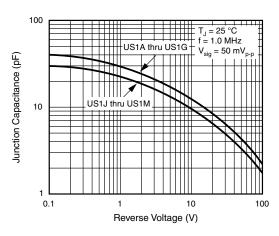
Fig. 7 - Typical Junction Capacitance
