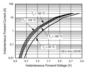
Fig. 5 - Typical Instantaneous Forward Characteristics
