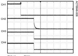
CH1: V<sub>PWRHLD</sub>, 2V/div CH2: V<sub>OUT4</sub>, 2V/div CH3: V<sub>OUT5</sub>, 1V/div CH4: V<sub>OUT11</sub>, 2V/div TIME: 1ms/div
