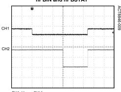
$\begin{array}{l} \text{CH1: V}_{\text{nPBIN}}, \, 2\text{V/div} \\ \text{CH2: V}_{\text{nPBSTAT}}, \, 2\text{V/div} \\ \text{TIME: } 10\text{ms/div} \end{array}$
