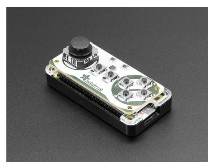
Once you get the Flash Complete! screen in Etcher, go ahead and remove the micro SD card from the reader and install in your Pi Zero (there is an opening in the case to slide it in).
