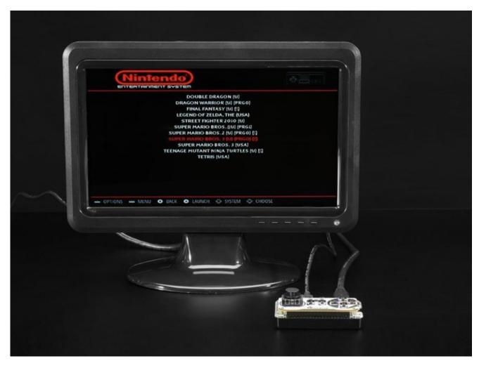
First, install the micro SD card into the Raspberry Pi Zero. Then, plug in the HDMI cable to a monitor or TV. You will need to use the mini HDMI side of the cable on the Raspberry Pi Zero, and the full size HDMI for your TV or monitor. Now, use the included power adapter and plug it in to the 'PWR IN' port on the Raspberry Pi Zero.
