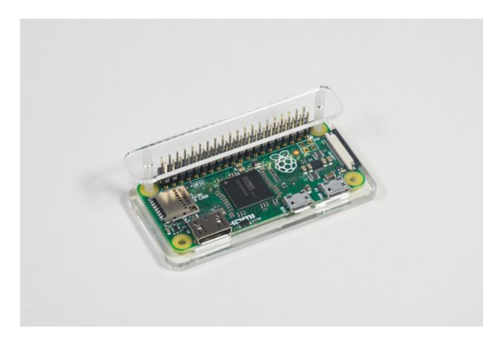
Using a hammer, gently tap back and forth on the top acrylic piece to push the pins through. Pushing one end of the header all the way it can cause the other pins to bend when you hammer them in. It's worth taking your time over this part.
