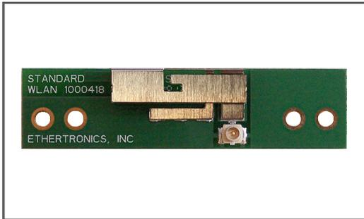
Ethertronics' Prestta series of Isolated Magnetic Dipole™ (IMD) stamped metal antennas address the challenges facing today's product designers. IMD's high performance and isolation characteristics offer better connectivity and minimal interference.
