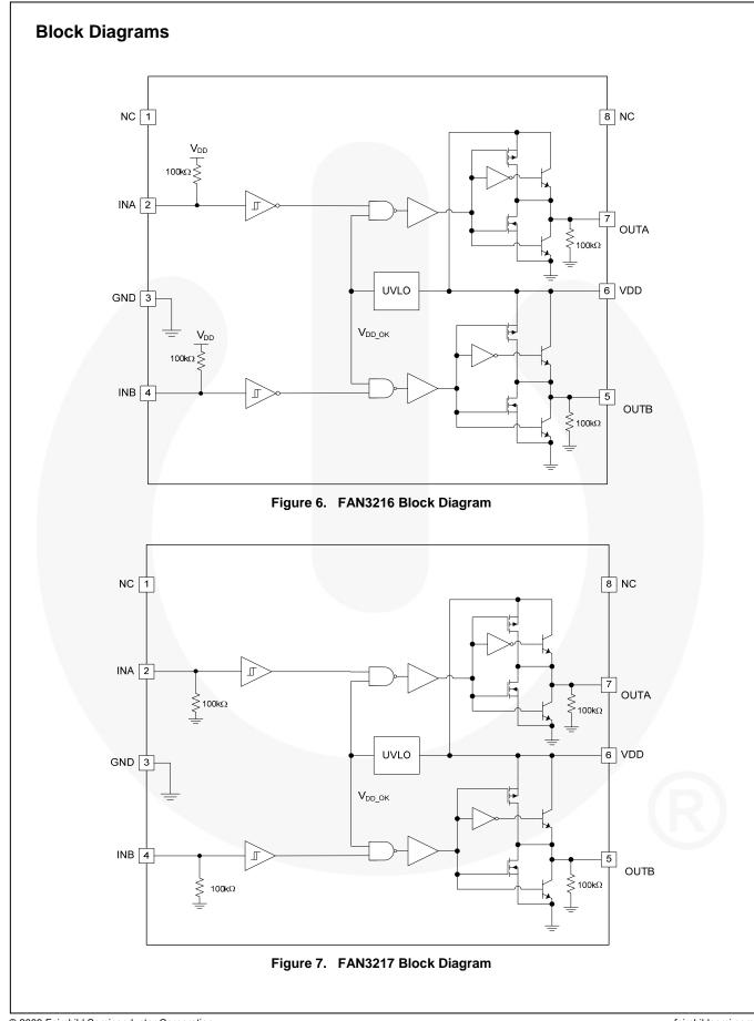
FAN3216 / FAN3217 — Dual 2-A, High-Speed, Low-Side Gate Drivers
