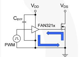
Figure 33. Current Path for MOSFET Turn-Off
