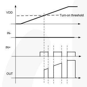
Figure 34. Non-Inverting Startup Waveforms
