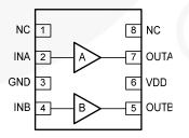
Figure 2. FAN3217 Pin Configuration
