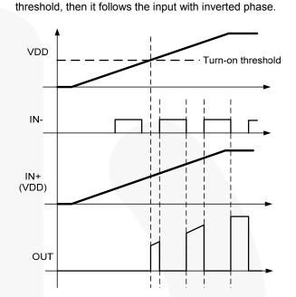
The inverting configuration of startup waveforms are
