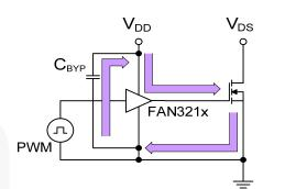
Figure 32. Current Path for MOSFET Turn-On
