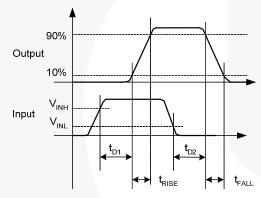
Figure 8. Non-Inverting Timing Diagram
