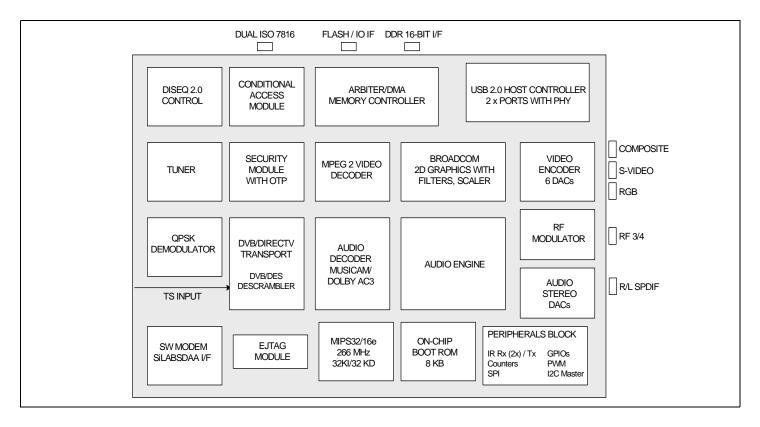
The BCM7312 is Broadcom's third-generation satellite set-top box system on a chip design, but it is the first to fully integrate the DBS Tuner. This is the first truly integrated single chip for DBS applications.
