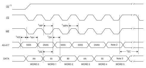
Notes: 1.  $\overline{OE}$  must be high only when  $\overline{WE}$  and  $\overline{CE}$  are both low.
