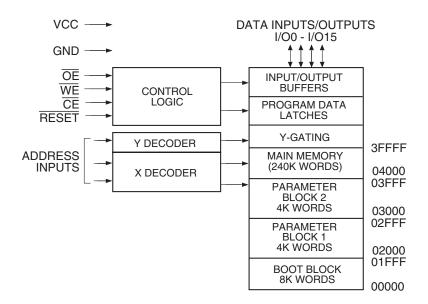
**Device Operation READ:** The AT49BV/LV4096A is accessed like an EPROM. When  $\overline{CE}$  and  $\overline{OE}$  are low and  $\overline{WE}$  is high, the data stored at the memory location determined by the address pins is asserted on the outputs. The outputs are put in the high-impedance state whenever  $\overline{CE}$  or  $\overline{OE}$  is high. This dual-line control gives designers flexibility in preventing bus contention.
