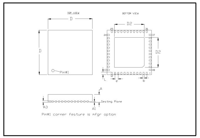
Note: The control dimension is in millimeter.
