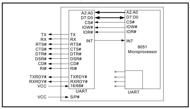
In the serial mode, the external serial port will need to communicate with the UART via AT commands.
