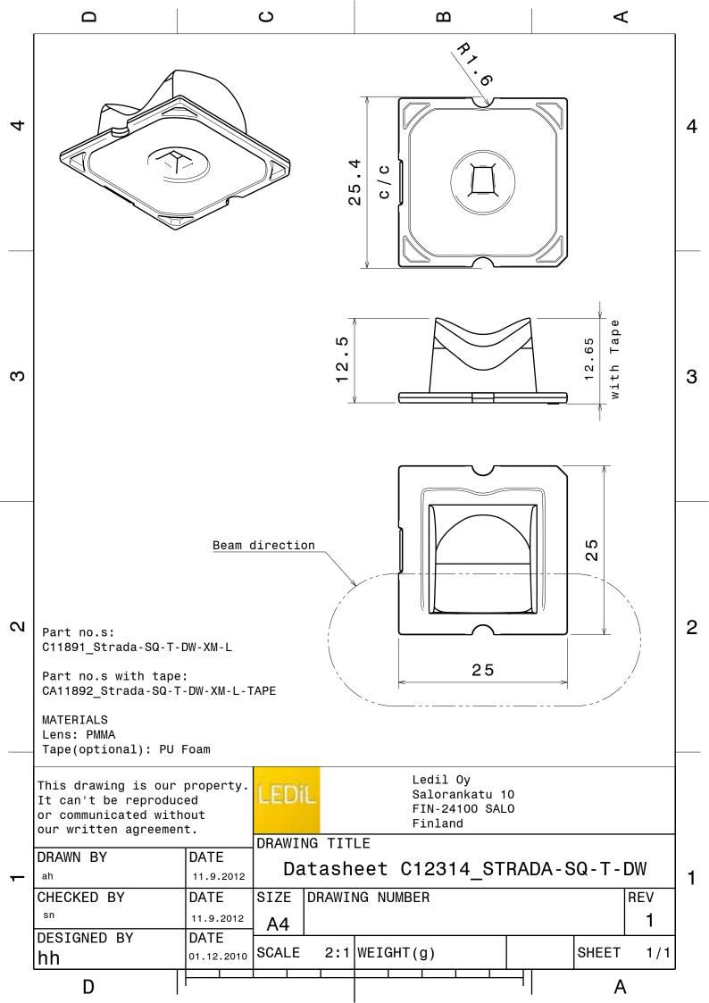
Luminaire: Ledil Oy C12314\_STRADA-SQ-T-DW/CA12312\_STRADA-SQ-T-DW (Cree XM-L 111Im @ 250mA) Efficiency=94% Lamps: 1 x Cree XM-L 111Im @ 250mA
