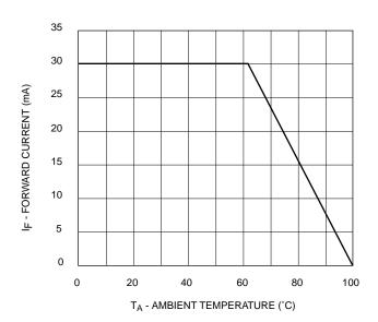
Fig. 5 Current Derating Curve
