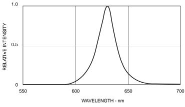
Fig. 3 Relative Intensity vs Peak Wavelength
