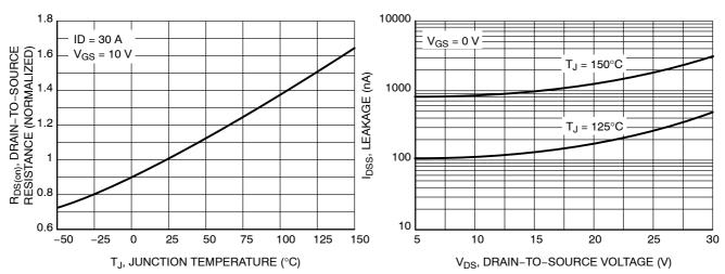
Figure 5. On-Resistance Variation with **Temperature**
