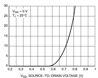
Figure 10. Diode Forward Voltage vs. Current
