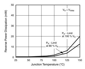
Fig. 4 - Max. Reverse Power Dissipation vs. Junction Temperature
