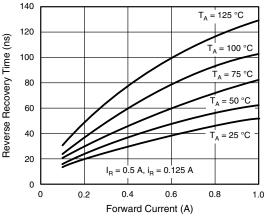
Fig. 6 - Max. Reverse Recovery Time vs. Forward Current
