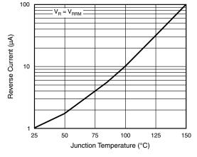
Fig. 3 - Reverse Current vs. Junction Temperature
