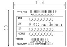
The LEAD FREE \* description shows that the surface treatment of the terminal is lead free.
